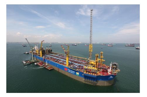
Hull conversion was concluded at the Keppel shipyard, in Singapore Topsides are already under construction at the BrasFels shipyard, in Brazil
